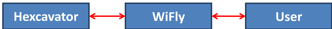
Figure 9: A flow chart demonstrating how the WiFly sends communications from the User in the command center to the Hexcavator and back.
