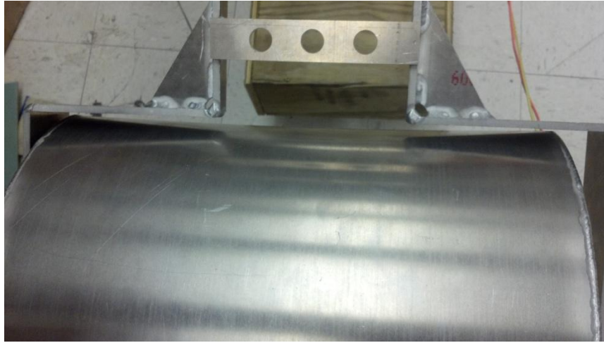
Figure 32: The edge of the drum and forked arm where more clearance could be added to mitigate a scraping concern.
