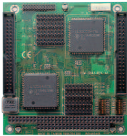
PCM-3643 4/8 RS-232 COM Port Module
